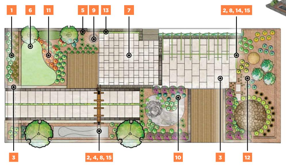
1 BIOSWALE DOWNSPOUT DISCONNECTION 2 3 DRAINAGE CHANNEL 4 DRY CREEK INFILTRATION PIT 5 LAWN AND LAWN ALTERNATIVES 6 PERMEABLE PAVEMENT 7 8 RAIN CHAIN 9 **RAIN BARREL** 10 **RAIN GARDEN** 11 RIGHT PLANT, RIGHT PLACE 12 SCREE GARDEN 13 SMART CONTROLLER 14 SOAKAWAY PIT **15** TREATMENT TRAIN
